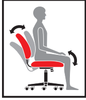
A TENSION ADJUSTMENT Increase or decrease to match body weight. Allows you to rock comfortably, without heavy pushing, reducing muscle fatigue.
