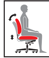
L SYNCHRO-TILT MOVEMENT Backrest reclines at a faster rate than the seat, increasing the angle between your torso and thighs. Enhances comfort and encourages dynamic body movement.
