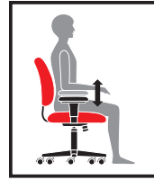
H ARM HEIGHT Adjust to support your forearms. Reduces muscular effort in neck and shoulders, minimizing risk of pain.
