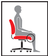
M WATERFALL SEAT EDGE Reduces pressure at the back of the knee, contributing to good blood flow.
