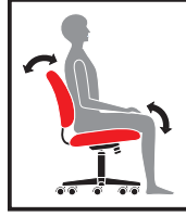
B CHAIR TILT LOCK Lock the tilt movement in position(s) to accommodate your working posture. Allows you to lock your chair in a comfortable and supportive position. (Can be either single position or infinite style.)
