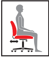
E SEAT DEPTH Change the depth of the seat to accommodate the length of your thighs. Keeps your back in contact with the backrest while avoiding pressure behind your knees.
